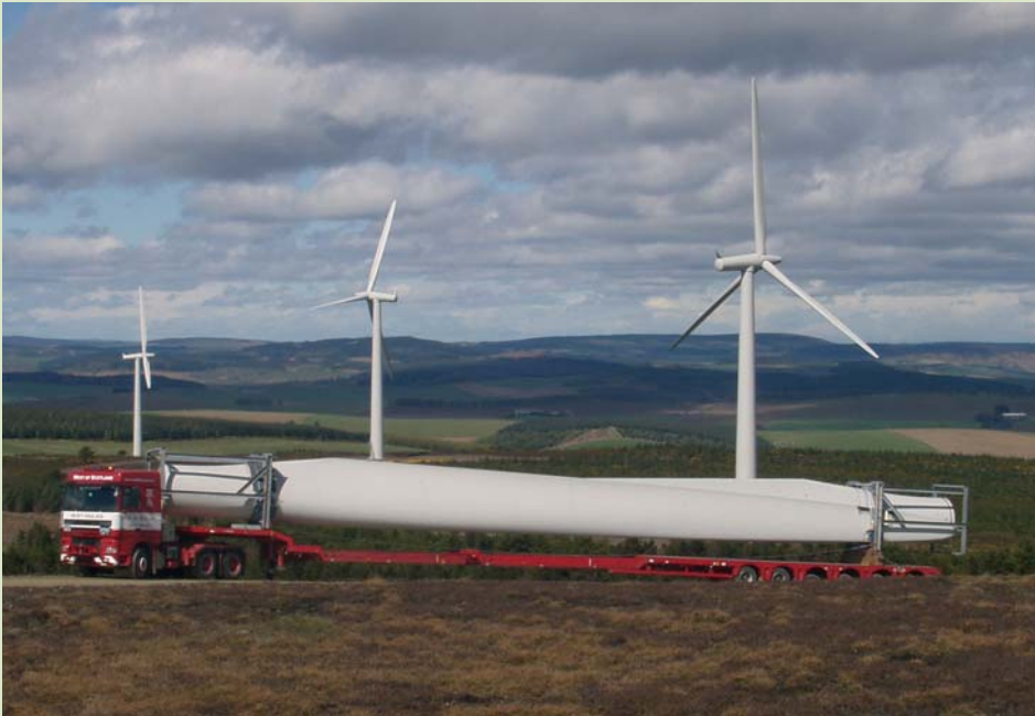
Wind turbine delivery vehicle at Glens of Foudland
